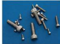
SOCKET SCREW Material: SUS304 A2 Size: M3—M24 3/16"—1" Length: 8mm—150mm Standard: DIN,ASME,ANSI
