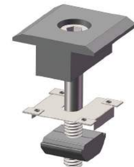
Ribs will penetrate module and rail andonization and create grounding path through rail
